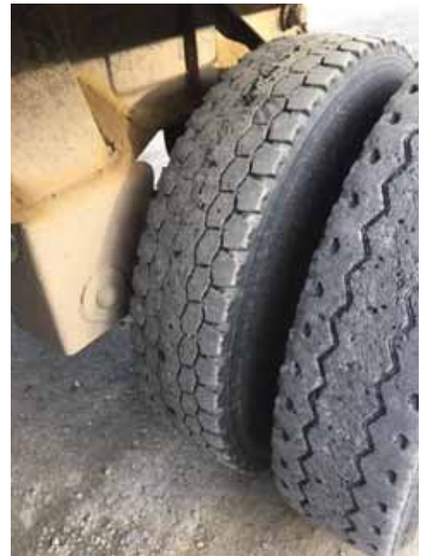
Worn out tires, steel cords showing. Photo by Ofc. Sheldon Barteaux, Whitehorse Weigh Station, Yukon, Canada.
