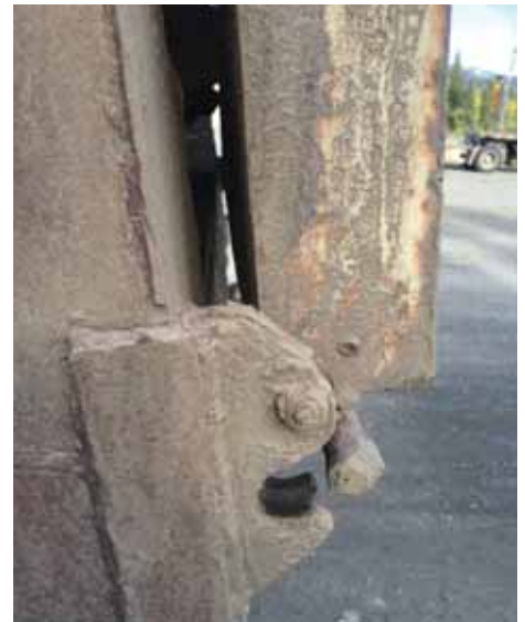
Broken latch on the back of an end dump trailer. Photo by Ofc. Sheldon Barteaux, Whitehorse Weigh Station, Yukon, Canada.
